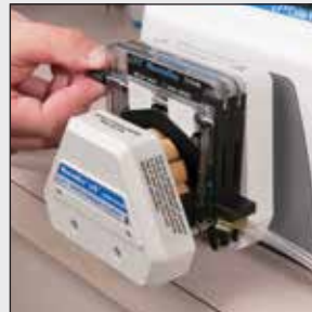
3. Adjust occlusion using index scale on cartridge.
